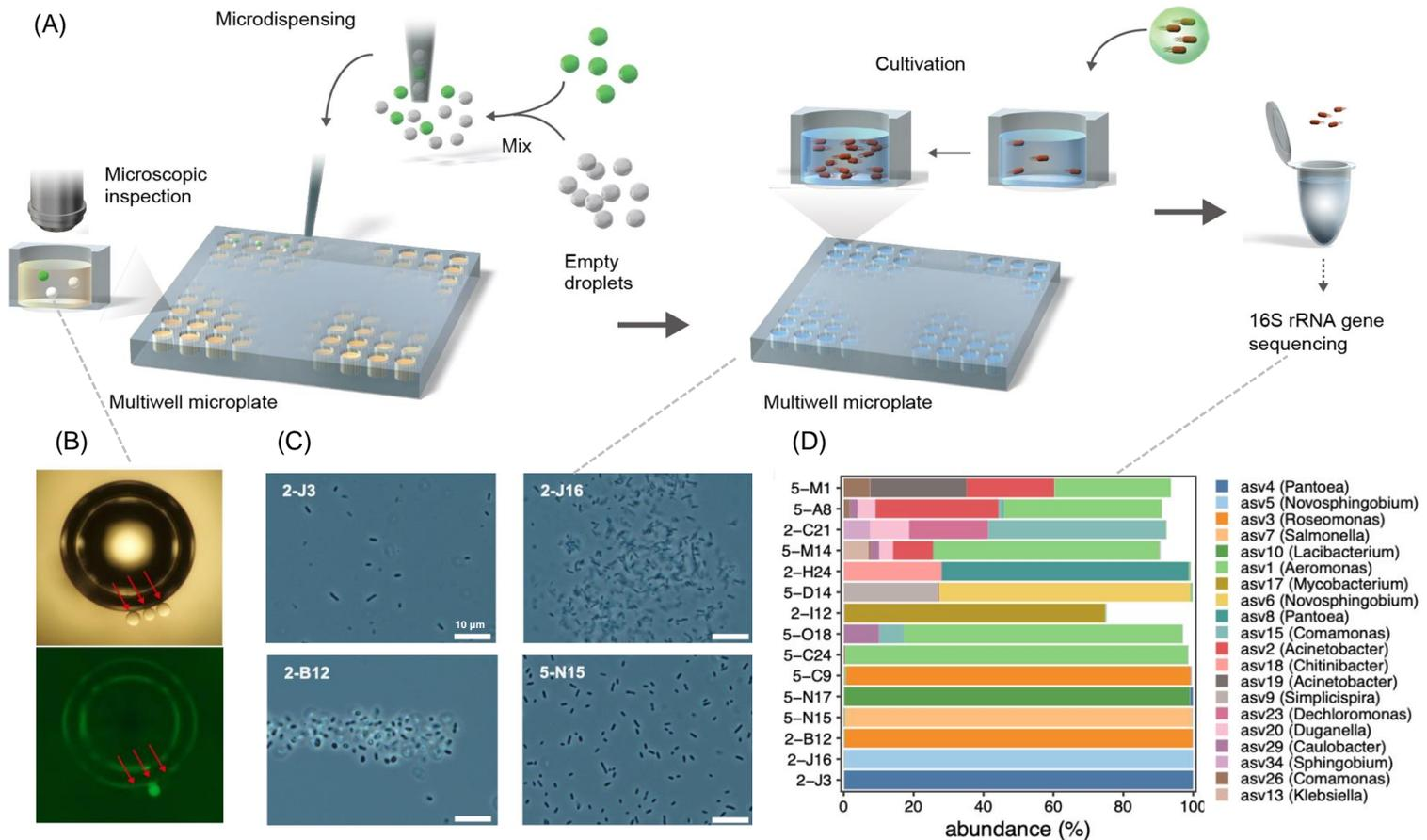
**Figure 1-3.** Droplet dispensing using On-chip SPiS and scale-up culture of microorganisms derived from individual droplets. (A) Droplet dispensing and analysis workflow, (B) microscopic images of dispensed droplets (upper panel: bright-field observation; lower panel: fluorescence observation), (C) microscopic images after scale-up culture of the dispensed droplets-derived microorganisms, and (D) microbiome analysis of the microorganisms in wells.
