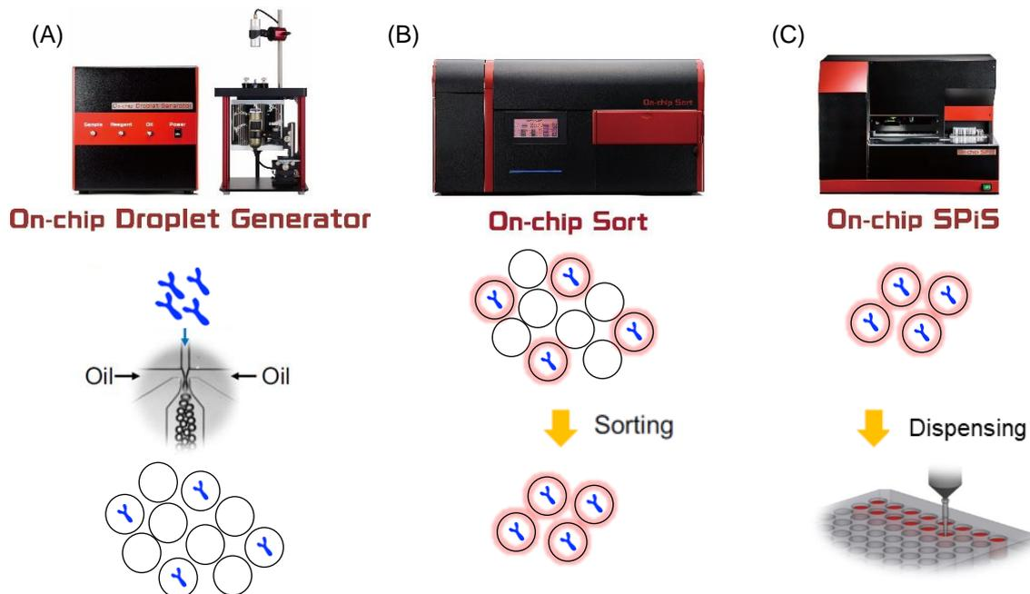
**Figure 7-1. Workflow for high-throughput screening of bifidobacteria using GMDs with On-chip Sort.** (A) Encapsulation of bifidobacteria into GMDs (a single cell per each one) with On-chip Droplet Generator, (B) fluorescent staining in GMDs and sorting with On-chip Sort, and (C) single cell (GMD) dispensing from sorted GMDs with On-chip SPiS.
