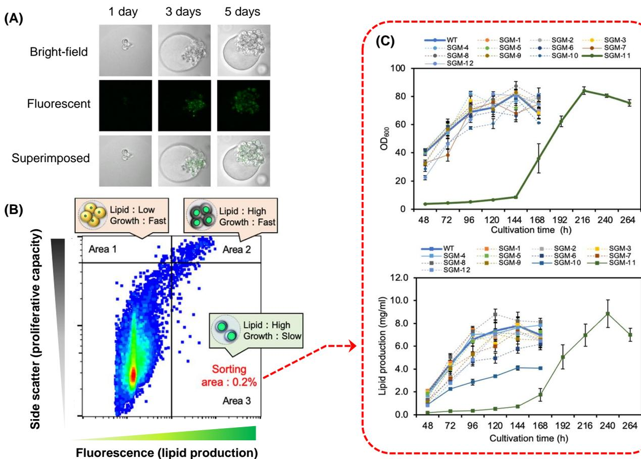
**Figure 6-1. Screening of oleaginous yeast using GMDs.** (A) Microscopic observation of GMDs containing cultured oleaginous yeast, (B) analysis of GMDs and sorting gate setting using growth and lipid-producing capacity of oleaginous yeast as indices, and (C) evaluation of growth and lipid-producing capacity of strains recovered from sorted GMDs.
