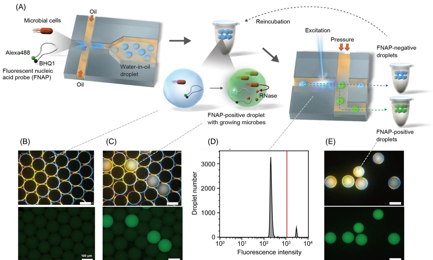
**Figure 1-1. FNAP-sort workflow and proof of principle.** (A) FNAP-sort workflow, (B) microscopic images of droplets immediately after generation, (C) microscopic images of droplets after one day of incubation, (D) fluorescence histogram of droplets after one day of incubation, and (E) microscopic images of sorted droplets. Upper panels: dark-field observation; lower panels: fluorescence observation for (B), (C), and (E).
