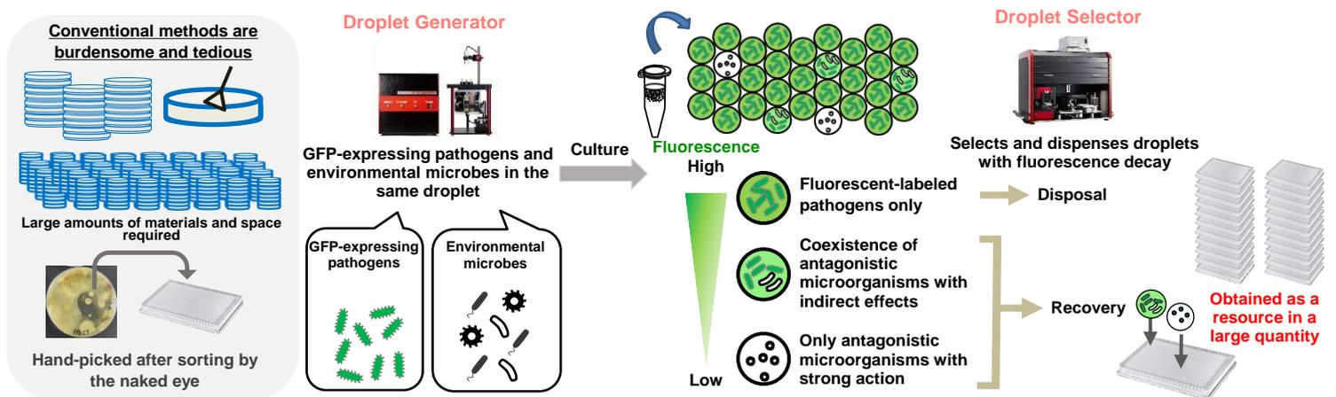
Figure 5-1. Workflow of the screening method for antagonistic microorganisms using droplet technology.
