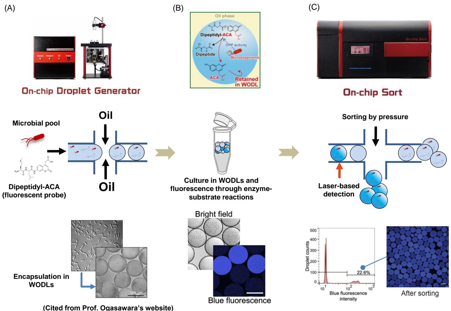
**Figure 2-1. Workflow for screening enzyme-producing microorganisms using On-chip Droplet Generator, dipeptidyl-ACA, and On-chip Sort.** (A) Generation of WODLs containing dipeptidyl-ACA and microorganisms using On-chip Droplet Generator, (B) an increase in fluorescence intensity due to microbial culture and DPP activity inside WODLs, and (C) detection of fluorescent WODLs using On-chip Sort and sorting-based recovery of microorganisms producing the enzyme at high yields.
