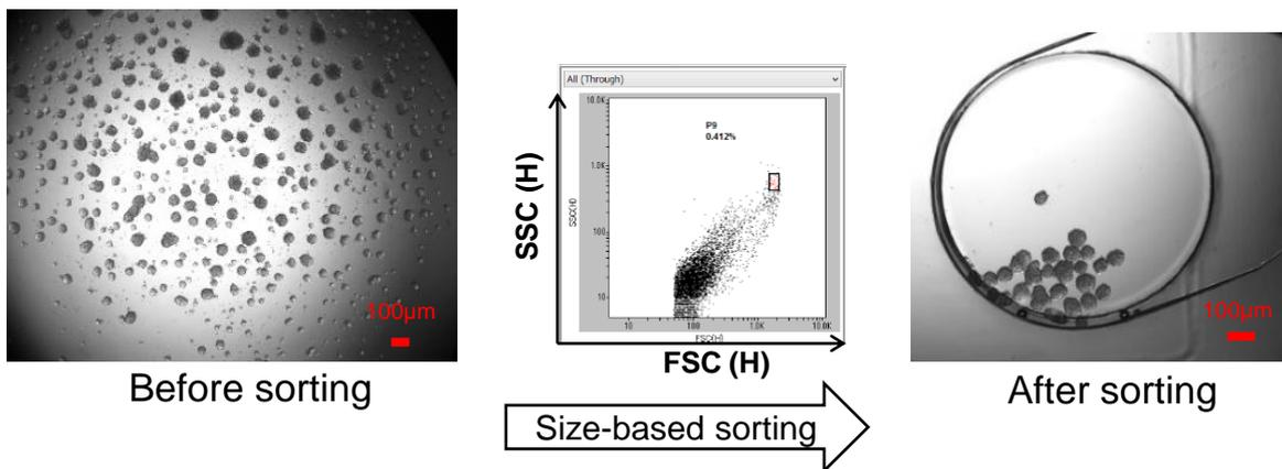
**Fig. 9** Sorting of 45  $\mu\text{m}$  spheroids using On-Chip Sort.
