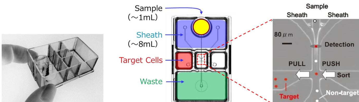
**Fig. 1** Our small and disposable microfluidic chip for analysis and sorting.
