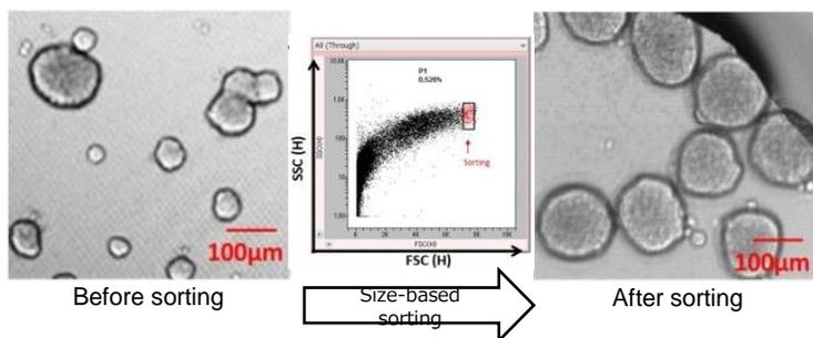
**Fig. 8** Sorting of 100  $\mu\text{m}$  spheroids using On-chip Sort.
