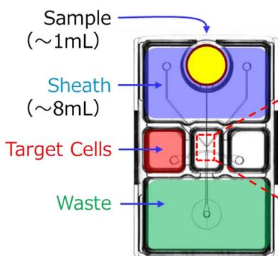
**Fig. 2** Reservoirs where initial sample, sheath fluid, waste liquid and collected sample are on the chip.
