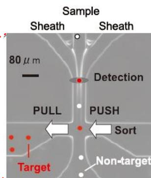
**Fig. 3** Enlarged image of sorting area of the chip and the Flow shift sorting mechanism.
