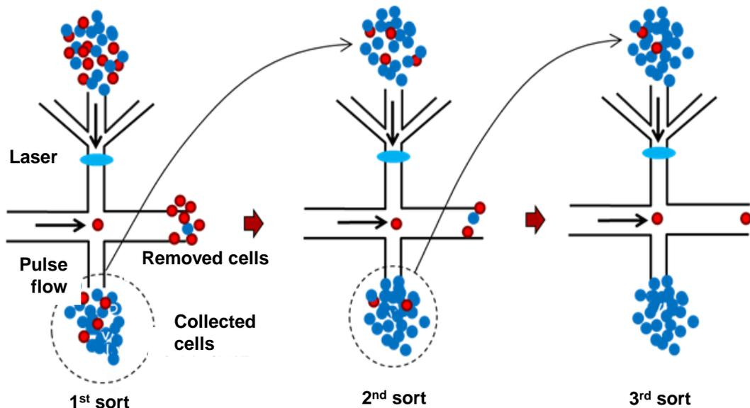
**Fig. 11** Principle of multi-step negative sorting. Red dots are undifferentiated cells and blue dots are differentiated cells.
