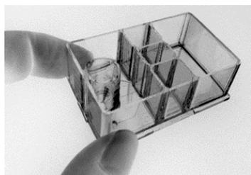
**Fig. 1** Our small and disposable microfluidic chip for analysis and sorting.
